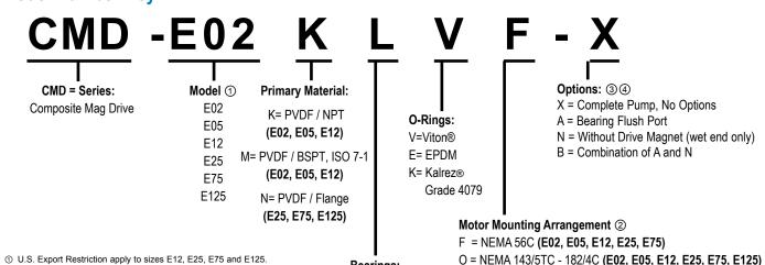
② Motor mounting flanges are available to order. Motors are ordered separately as a line item. Customer is responsible for motor mounting. Option O 182/184C motor requires modified motor shaft and motor bolt pattern. Does not fit frames 182/184TC
