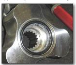
Install each rotor on shaft, making sure they are completely seated before installing rotor retainer screw.  Install rotor retaining screw and torque to 109 NM (80 lb ft). Grease o-ring located behind retainer.
