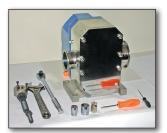
Remove rotor retaining screws (both right hand threads) using 15/16" or 24 mm socket. It may be necessary to block rotors from turning by using a soft object. Remove rotor; if rotor is difficult to remove, attach puller or similar tool to threaded holes in rotor to remove.
