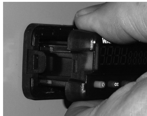
Grab the unit above and below the face and pull forward.
