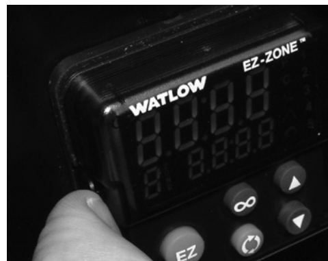
Pull out the tab on each side until you hear it click.
